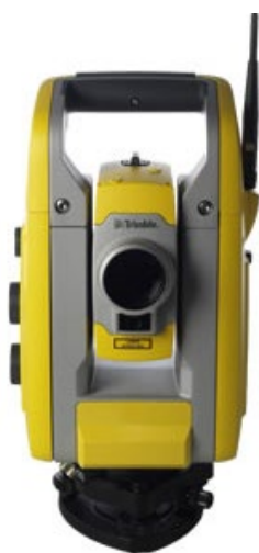
Figur 5.15. En totalstation, Trimble S3.
